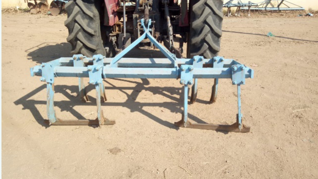
Tractor operated twin blade for intercultivation in cotton
