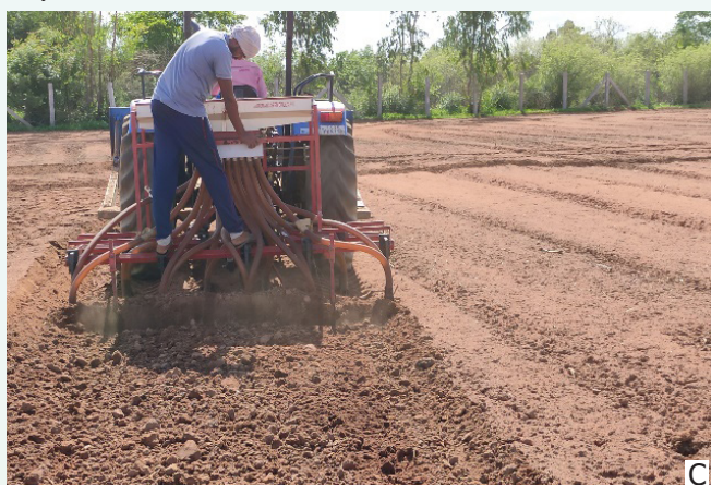
Sowing and basal dose fertilizer application in cotton using seed cum ferti drill
