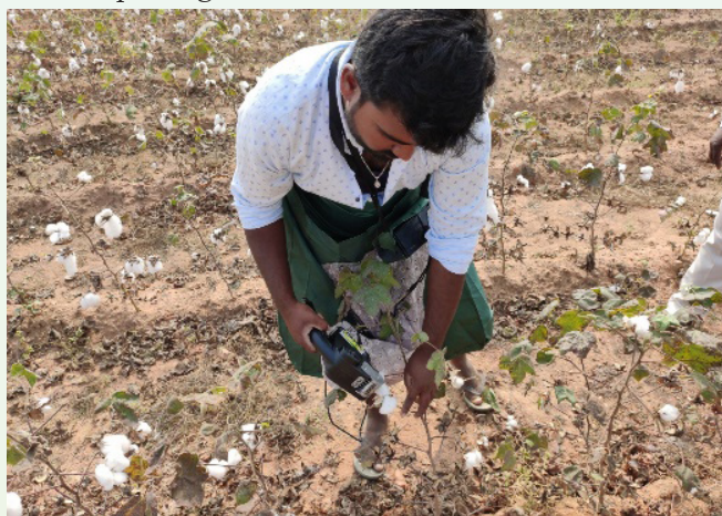
Field operation of Hand held battery operated cotton-picking machine
