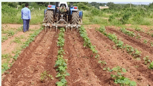
Intercultivation in cotton with tractor operated cultivator
