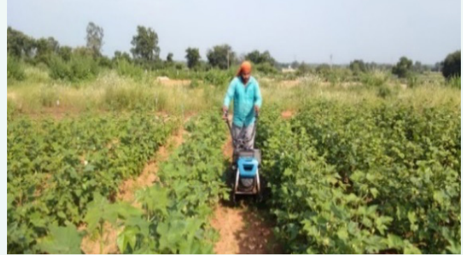
Intercultivation in fully grown cotton with power tiller
