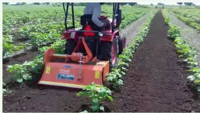
Intercultivation in cotton with mini tractor operated rotavator
