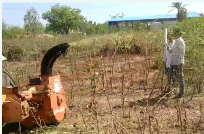
Tractor operated multi-crop shredder for chaffing cotton stubbles
