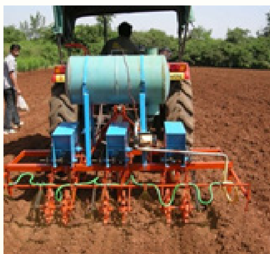
Figure 2: Sowing pigeon pea with high precision plater cum herbicide applicator
