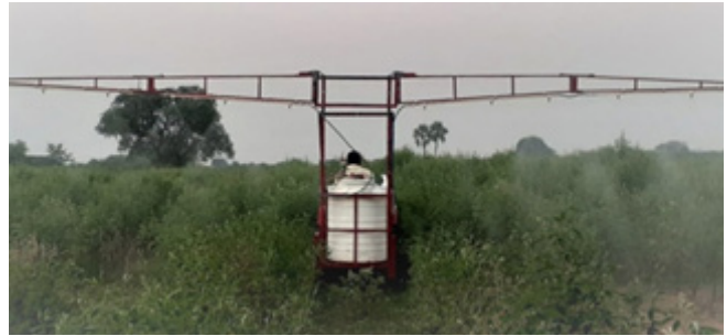
Figure 8: Spraying with tractor mounted boom sprayer
