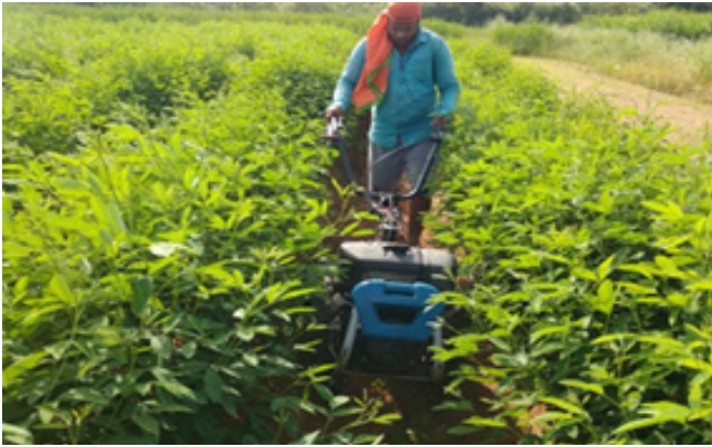
Figure 5: Intercultivation with power tiller at later stage of pigeon pea
