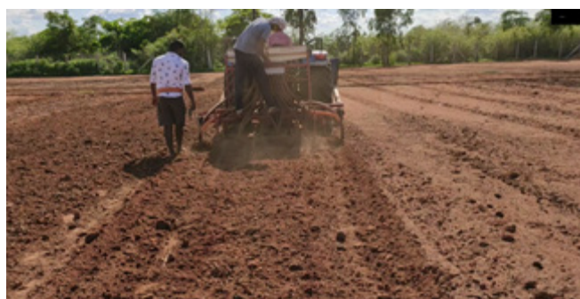
Figure 1: Sowing pigeon pea with seed cum ferti drill
