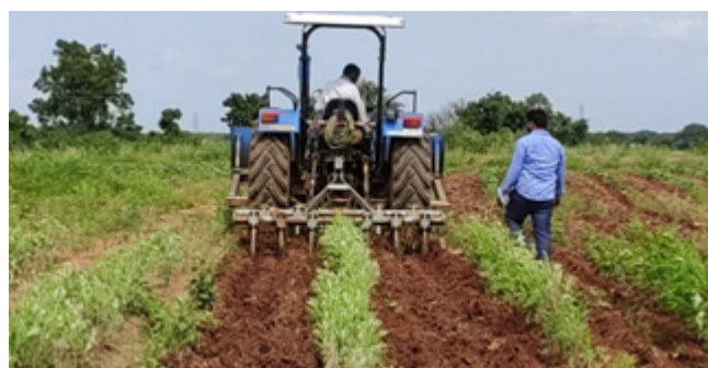
Figure 3: Intercultivation with tractor drawn cultivator in early stages of pigeon pea
