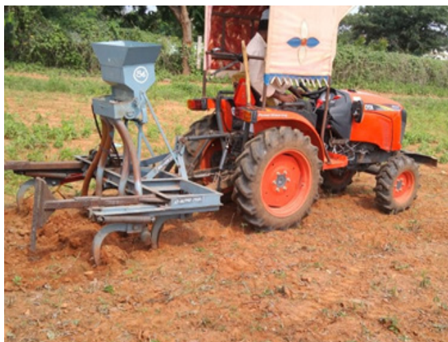
Figure 3: Small/ Mini tractor (25 HP) operated automated Ananta planter suitable for strip cropping
