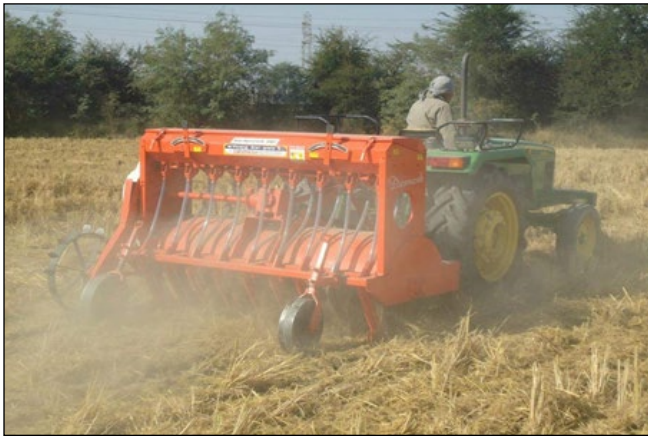
Figure 6: Use of 'Happy Seeder' for direct sowing of seeds
