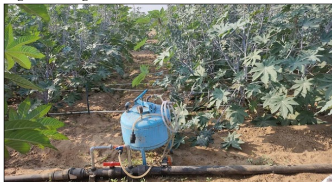
Figure 3: Field view of installed drip system with fertigation unit
